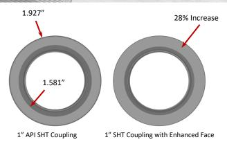
design fosters consistent circumferential displacement (CD) and preload stress values during makeup, helping to reduce connection related failures. In addition, all couplings are furnished with cold formed threads that provide additional strength and fatigue resistance. All LUFKIN couplings are manganese phosphate coated
