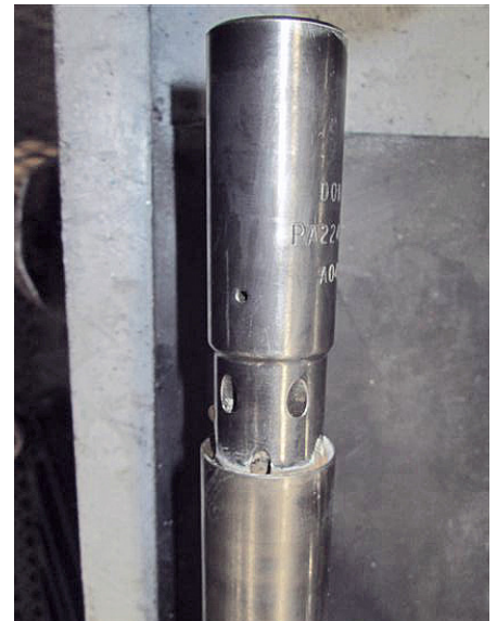
A plunger with a standard plunger adapter (top) shows extreme abrasion after only 100 days in operation, making it unacceptable for redeployment. A plunger fitted with a Sand Diverter plunger adapter (bottom) shows no signs of plunger abrasion damage after 226 days in operation and can be redeployed.
