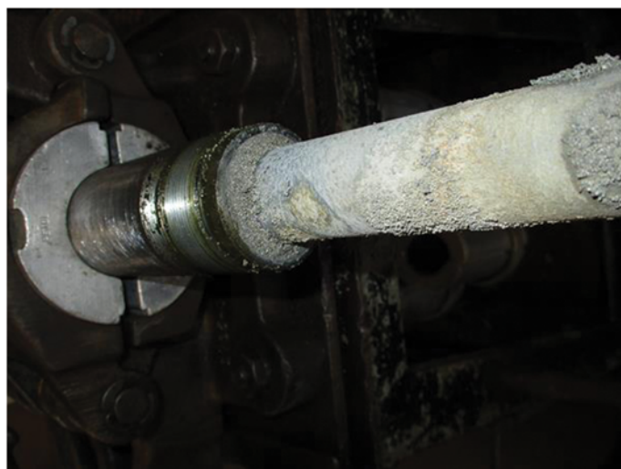
Image 2: SRP travel assembly stuck in standing assembly due to solids, observed during disassembly.
