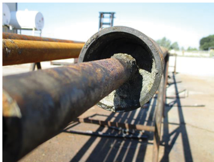
Image 1: SRP stuck in tubing due to solids
