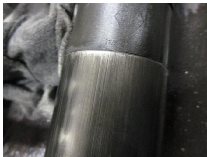
Image 2: Plunger spray metal grooved from formation solids.
