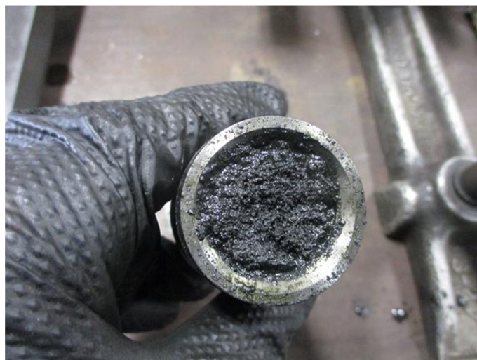
Image 1: Travel valve cage packed off with formation solids.
